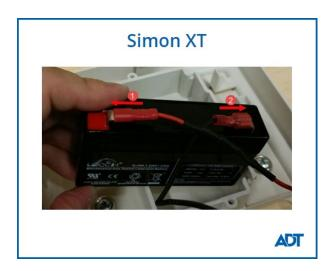
4. Insert the new battery into the battery compartment with the terminals at the bottom. Tuck the wires underneath the bottom retaining clip. Snap the battery into place between the retaining clips.
